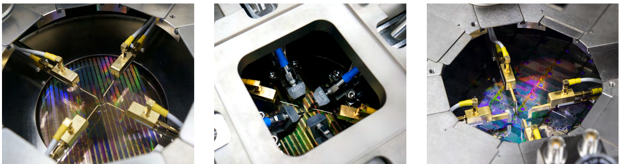
Typical MPI configuration with Kelvin Probes
