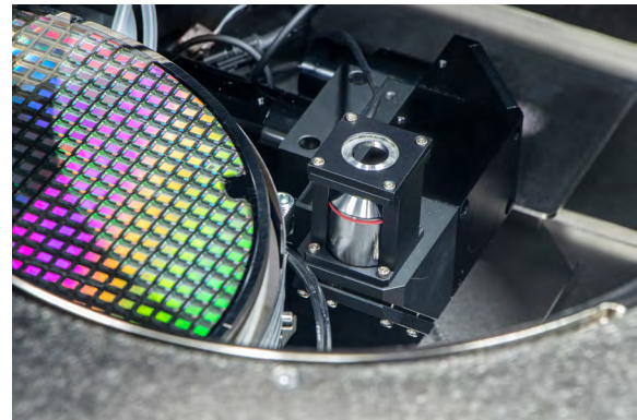
Optional upper looking chuck camera for probe-to-pad alignment
