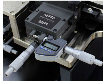
The MP80-DX MicroPositioner with the digital micrometer on the X axes.
