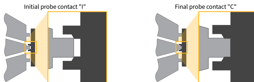
Figure 6. Image shows correct alignment and placement of TITAN™ RC Probe with optional Reduced Contact 20 \mu\text{m} probe tip width.
