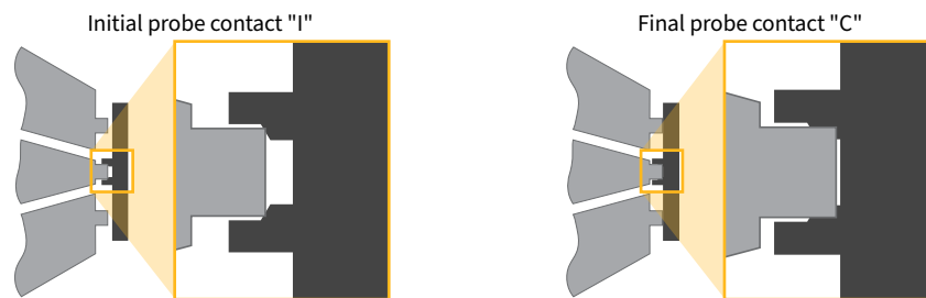
Figure 5. Image shows correct alignment and placement of TITAN™ Probe with standard 30 \mu\text{m} probe tip width.
